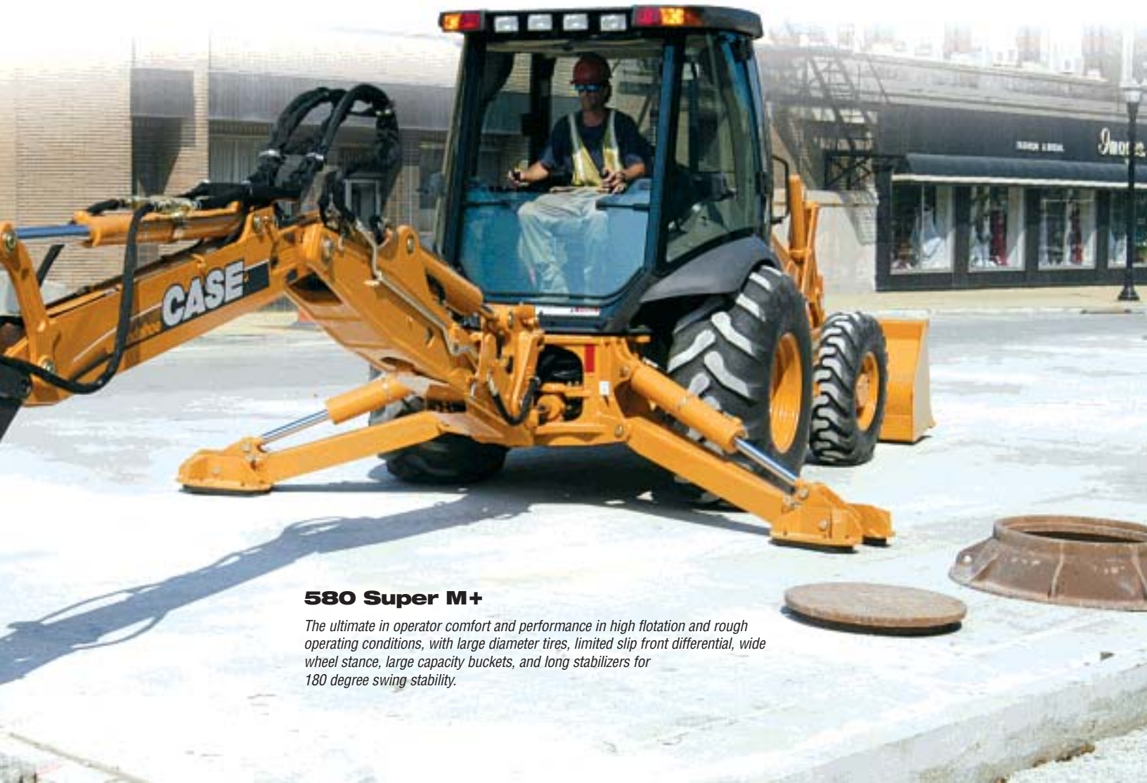
The versatile loader backhoe that delivers extra horsepower for high altitudes and contractors needing increased loader and transport speed.
